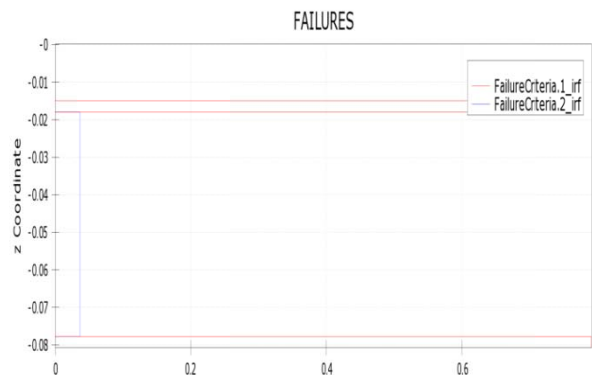
Fig. 13: Tsai-Wu Inverse Failure Factor for Sandwich Layup Configuration
